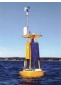
EMM2000 Coastal Monitoring Buoy
