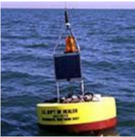
EMM700 Water Quality Monitoring Buoy
